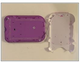
Using the iFixit opening tool, pry off the purple and white child-proof casing to expose the twelve screws.
