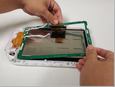
Unscrew the eleven 7.0 mm Phillips #1 screws securing the circuit board to the case. Remove the circuit board.
