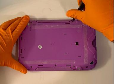
Remove all twelve 7mm Phillips #1 screws located along the edges of the device.
