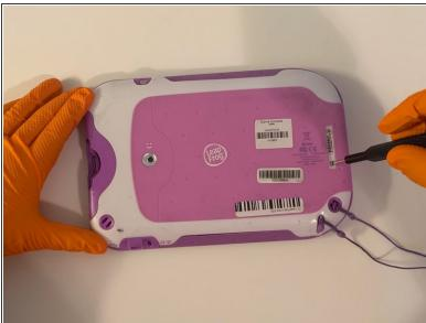
Remove the two 5.0mm Phillips #0 screws.
