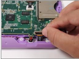
• Unscrew the four 5.0 mm Phillips #0 screws securing the motherboard.
