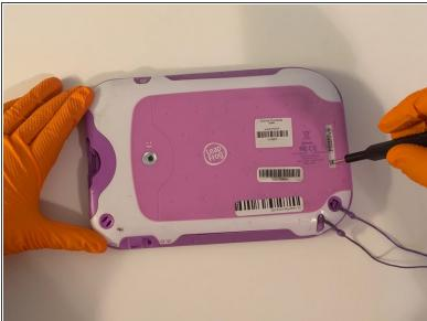
Remove the two 5.0mm Phillips #0 screws.
