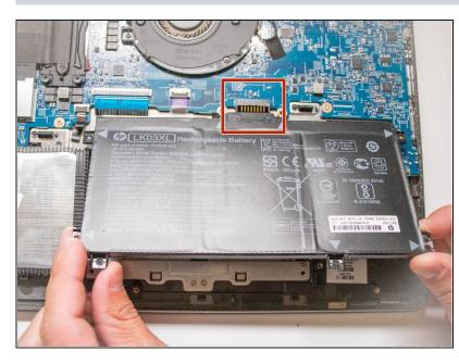
Lift and pull the front of the battery up and out (away from the connector) to remove.
