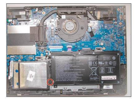
Using the Philips #0 screwdriver, remove the final screw from the battery connected to the SSD storage unit.
