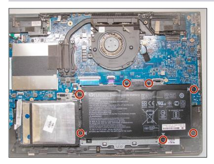
Use the Philips #0 screwdriver to remove six (6) M2.0x3.2 screws from battery.
