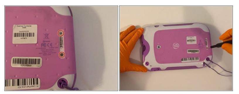
Remove the two 5.0mm Phillips #0 screws.
