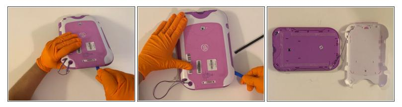
Using the iFixit opening tool, pry off the purple and white child-proof casing to expose the twelve screws.
