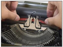
• Thread the ribbon into the ribbon vibrator.
