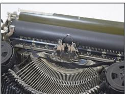
• Un-thread and remove the ribbon from the ribbon vibrator.
