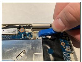
Disconnect the charging connector from the motherboard using the blue iFixIt opening tool by sliding it away from the connector.
