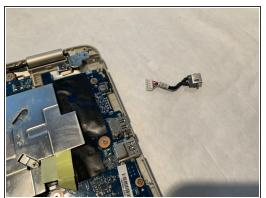
Pry the power connector upwards from the side of the laptop using the opening tool, then remove the part from the laptop.
