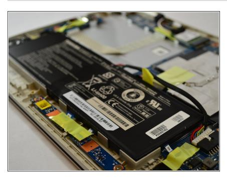
Remove the 1" yellow tape on top of the battery. This piece of tape is holding down the battery connection cable.
