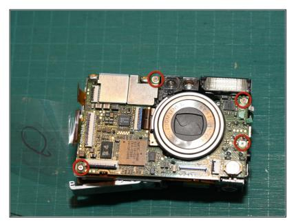
Remove the 4 screws holding the main logic board to the rest of the camera.
