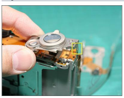
The shutter button can be removed by simply releasing the 2 small catches (one outlined with a yellow square, the other hidden by my thumb)
