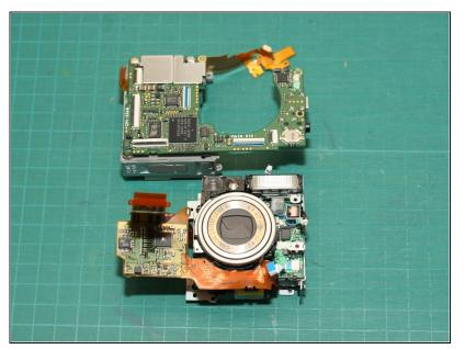
Here's a view of the lens module/viewfinder/flash assembly (bottom) separated from main logic board/battery compartment (top)
