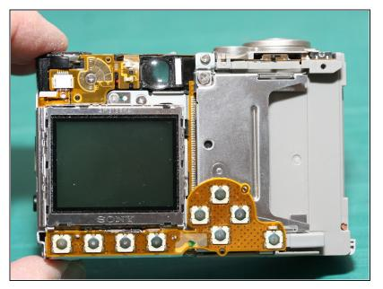
Here is the back of the camera without the shell. You can see the switch contacts on the flex circuit along the bottom.
