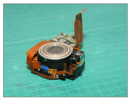
Here's a view of the lens module after removing the flash module. That's the optical viewfinder towards the right of the unit.
