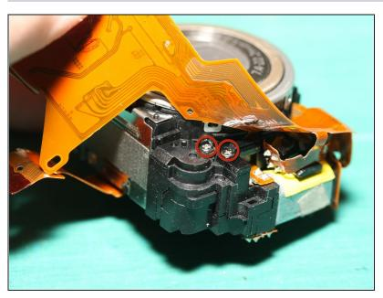
These 2 screws need to be removed before separating the lens module front and back halves.
