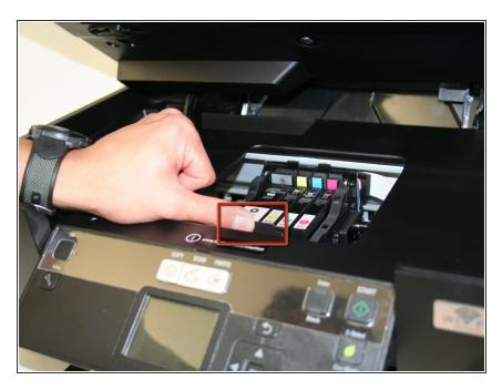
Locate the frame around the ink cartridges. Press the button located at the front of the cartridge frame.
