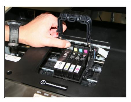
Lift the frame to expose the ink cartridges.
