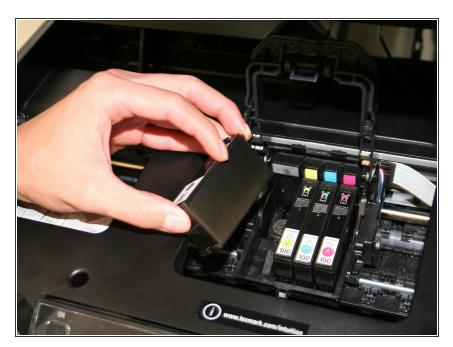
Pull the cartridge out, and place the new ink cartridge back into the slot.
