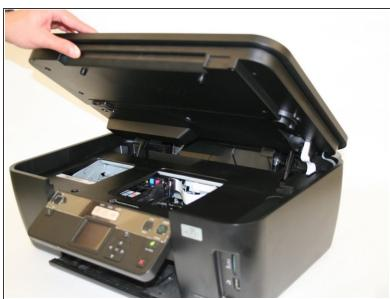
Lift the scanning unit, exposing the print head.
