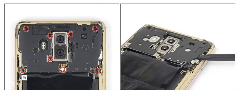
(i) The next two steps show how to remove the heat dissipation layer, along with its plastic bracket.
