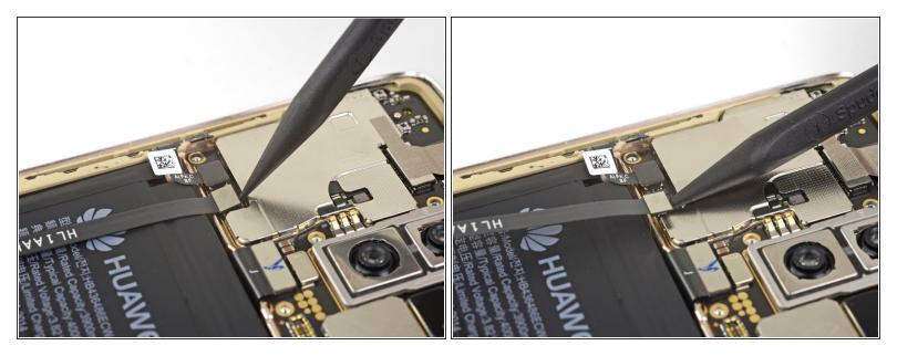
Use the point of a spudger to pry up and disconnect the fingerprint extension cable from its motherboard socket.
