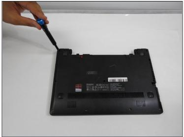
Using the #0 Phillips screwdriver, remove the nine 4mm screws on the back panel.
