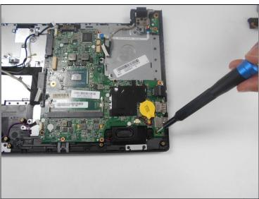
• Using a #0 Phillips screwdriver, remove the seven 3mm screws securing the motherboard to the chassis.
