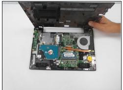
• Slowly begin working your plastic opening tool along the panel to undo the latches around the laptop.
