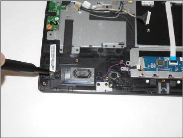
Using a #00 Phillips screwdriver, remove four 1mm screws from the two speakers.
