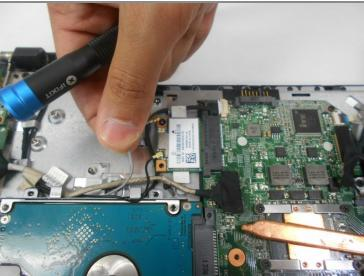
• Remove both antenna wires by pulling upwards gently.
