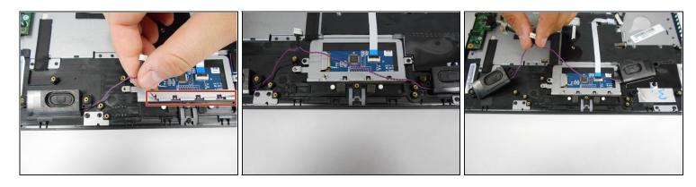
Separate the wires from the chassis and lift to remove the speakers.
