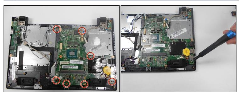
• Using a #0 Phillips screwdriver, remove the seven 3mm screws securing the motherboard to the chassis.
