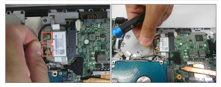
• Remove both antenna wires by pulling upwards gently.
