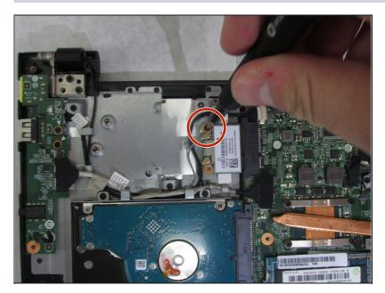
• Using the #00 Phillips screwdriver, remove one 3mm screw from the network card.
