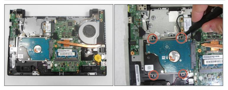
• Using a #0 Phillips screwdriver, remove the four 4mm screws that secure the hard drive bracket to the motherboard.
