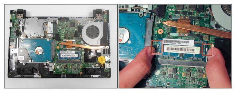
• Release the RAM from the motherboard by pressing the two locking latches away from each other.
