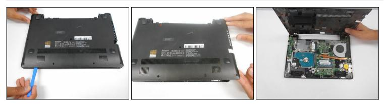
• Slowly begin working your plastic opening tool along the panel to undo the latches around the laptop.
