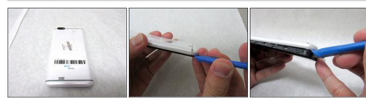
• With the phone face down, remove the back cover with the plastic opening tool. For easiest access, insert the plastic opening tool in the bottom left corner.
