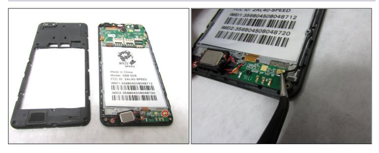
• Locate the wire that attaches the motherboard to the daughter-board of the speaker and mic. Using <u>tweezers</u>, disconnect the wire from the motherboard.
