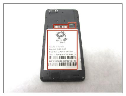
After the back cover is removed, remove the battery, sim cards, and micro SD card. These components are highlighted in red.
