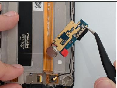
Use the tweezers to gently pull up on the bottom of the chip that houses the charging port.
