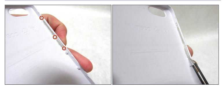
• There are three areas holding the power and volume buttons in place. Gently pull the bottom of the power button with a pair of fine-tip <u>tweezers</u> to release the lower half.
