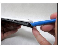
• Remove the back cover by gently prying open the bottom left corner of the case with the plastic opening tool.
