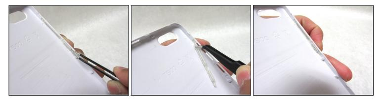
• Carefully remove the top section of the button with the fine-tip tweezers . This should free the button completely.
