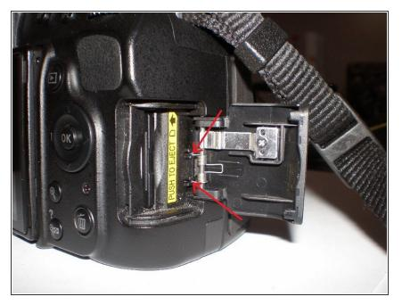
FIRST: open the memory card door and take a good long look at how the spring is installed. There are two "feet" coming off of the spring that need to be installed into two "insets" on the rear camera cover, this has to be done before you put the cover back on.
