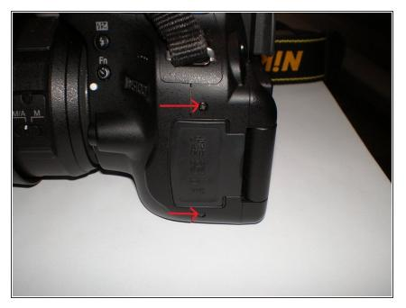
• Remove 2 long screws from the left side of the camera.
