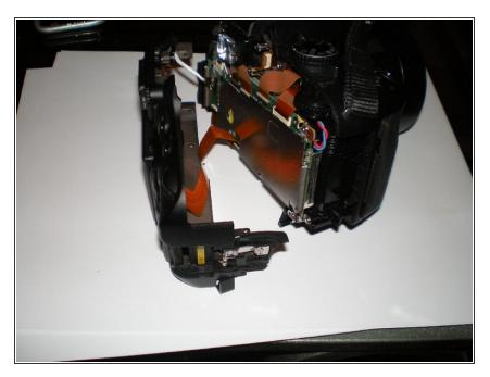
Once you remove those screws (12 altogether) you can pull the back cover off the camera, it is still attached to the camera body via two cables so be careful not to damage them. You will then see that the memory card door slides right out between the rear cover and the camera body.
