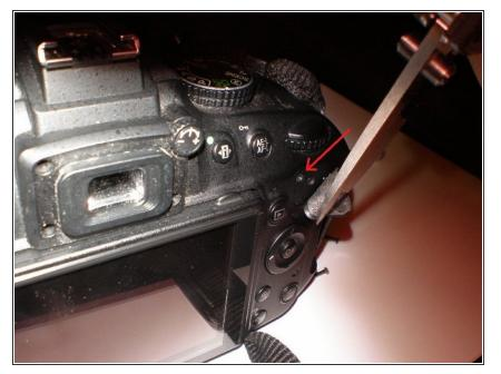
• Peel the rubber thumb-grip back slightly, there's a short screw there closest to the left side of the thumbgrip. This one seems to be slightly thicker than the ones in the next step, keep it separate.
