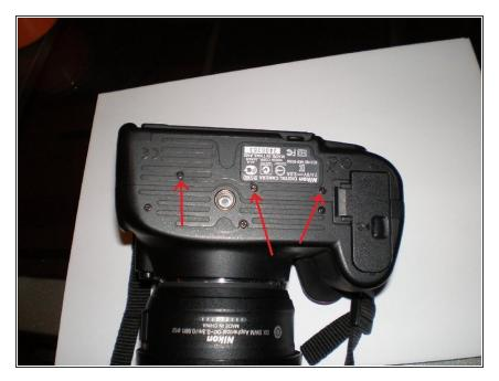
• Remove 3 short screws from the bottom of the rear cover.
