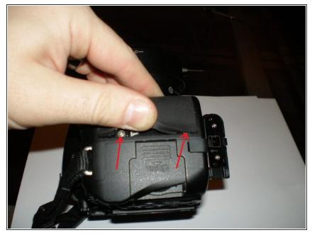
• Peel back the rubber grip on the right side of the camera, closest to the top and bottom behind the rubber grip there is a silver screw (2 total).
