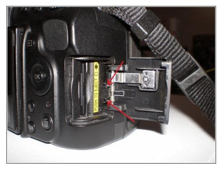
Install the new door making certain to put the spring back the way it was, with the two feet installed into the insets. Put the rear cover back on and test the memory card door to make sure it's working, then install all of the screws back where they went. Reapply adhesive to the rubber grips and diopter cover if desired.
