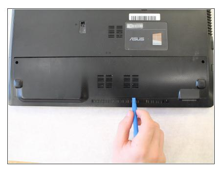
Using the iFixit opening tool, gently pry the plastic cover away from its original position.
