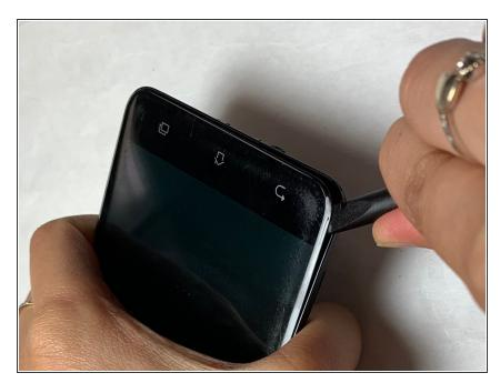
Progress around the perimeter of the phone with the pry tool till the screen is off.
