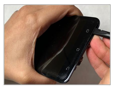
Pry off the screen beginning at the right-hand side toward the bottom of the phone with the plastic flat-edge spudger.
