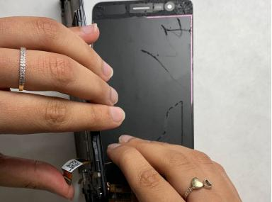
Remove the screen by pulling the attached ribbon cable out through the exposed opening.
