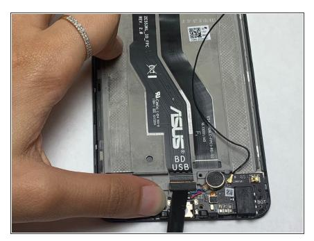
Gently pry off the ribbon cable from speaker housing with the flat-edge side of the iFixit plastic spudger.
