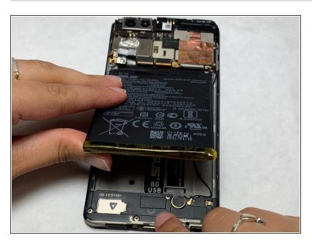
After removing the bracket and screws, pull up on the battery from the bottom of the unit and set aside.
