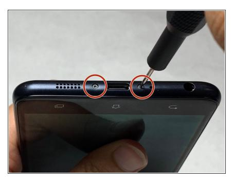
Remove the 3.5 mm screws on both sides of the charging port, at the bottom of the phone, using the T2 screwdriver.
