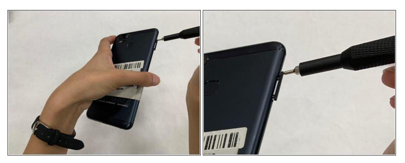
Use sim card attachment for the screwdriver found in the IFIXIT box to remove the sim card tray from the phone.
