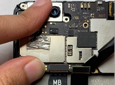
Use the flat-edge side of iFixIt plastic spudger to detach both of the ribbon cables off of the motherboard at their connection point.
