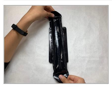
Use iOpener to soften the adhesive keeping the screen on the device.
