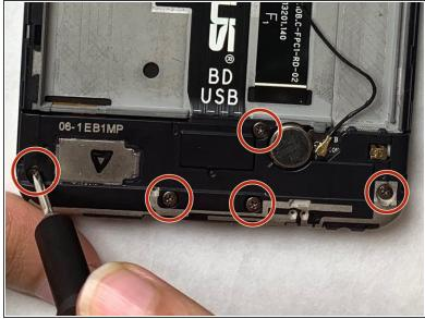
Remove the speaker cover at the bottom of the casing by taking out all five 3.25 mm screws with the PH #00.
