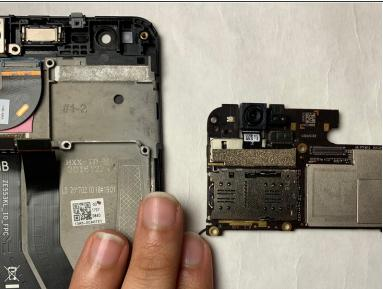
• Use the tweezers to lift up on the edges of the motherboard located above where the battery was, then remove the motherboard.
