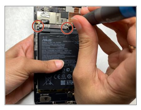
Utilize the PH #00 attachment to remove the two 3.3 mm screws in the bracket to the top left of the battery.
