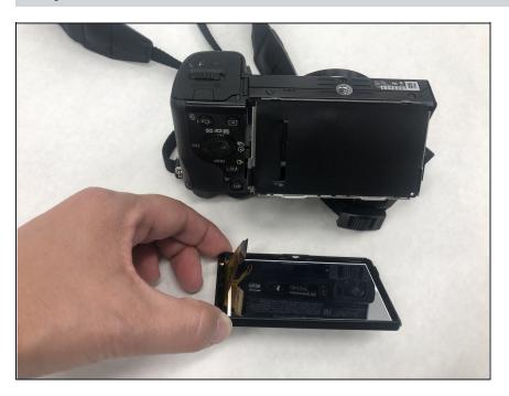
Pull the LCD screen away from the camera and set aside.
