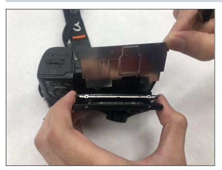
Remove the silver shield from the back side of the LCD screen.
