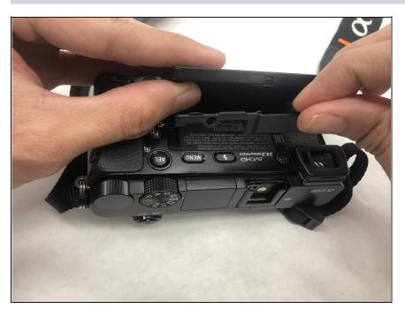
Remove the smaller bracket covering the bottom portion of the control board.
