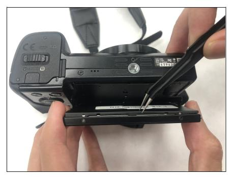
Carefully separate the bottom border of the frame from the back surface of the LCD screen.
