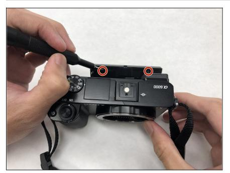
Remove the two 1.75mm Phillips #00 screws located on the back side of the LCD screen.
