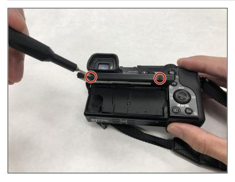
Remove the two 1.75mm Phillips #00 screws located on the bottom border of the LCD screen.
