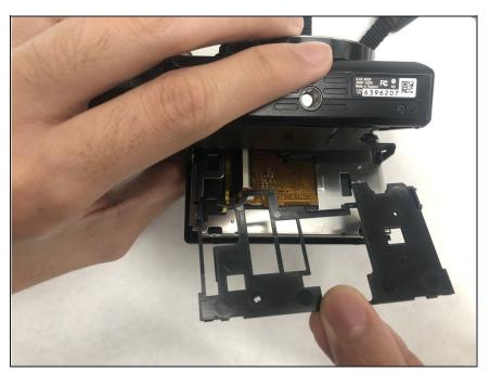
Carefully remove the spacer from behind the LCD screen.
