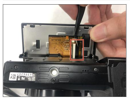
Detach the ribbon from the socket with a pair of tweezers.
