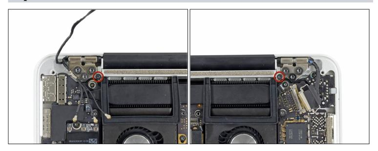
• Remove the two 3.1 mm T5 Torx screws securing the aluminum hinge brackets.
