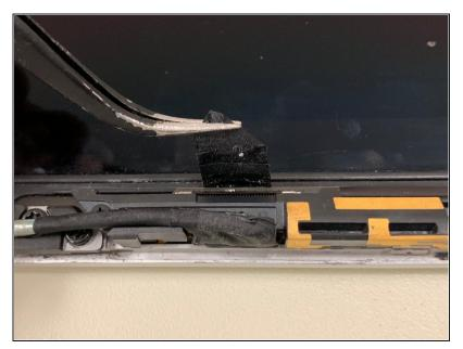
• Peel up the tape covering the cable connector.
