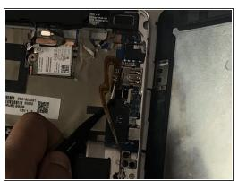
Detach flex cable from motherboard using tweezers.
