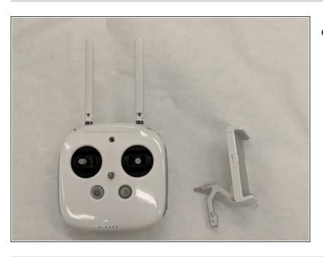
Replace the mobile device holder with a new one.
