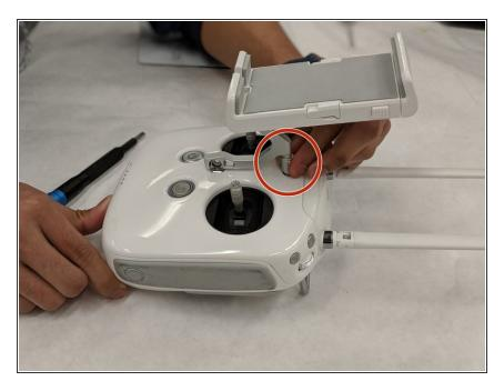
Loosen the bolt that is connected to the body by hand.
