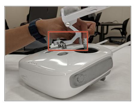
Lift up and disconnect the bracket from the body.
