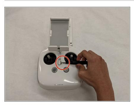
Remove the 6.7 mm Flathead screw using a Flathead 4 mm screwdriver.
