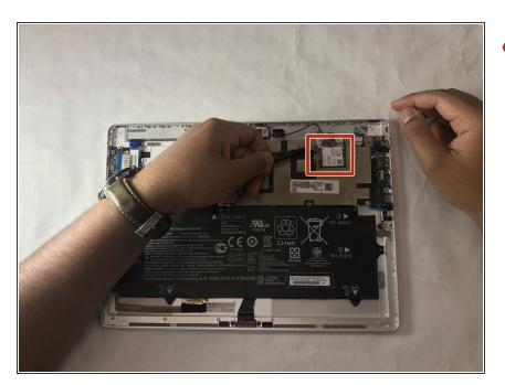
Detach the WWAN card from the motherboard by pulling it to the left using tweezers.
