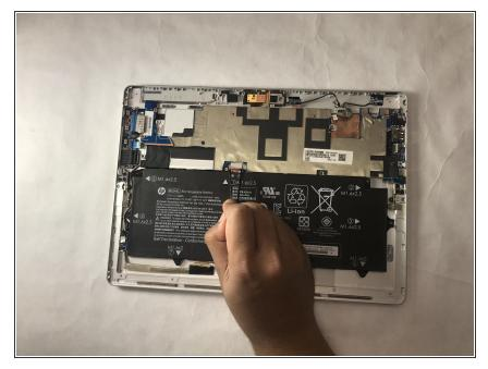
• Unplug the battery wire attached to the motherboard using tweezers.
