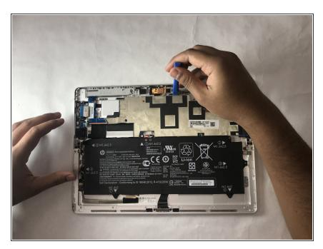
• Use the plastic opening tool to loosen the motherboard.
