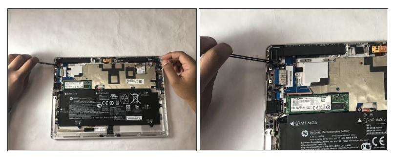
• Unplug the speaker wire attached to the motherboard.
