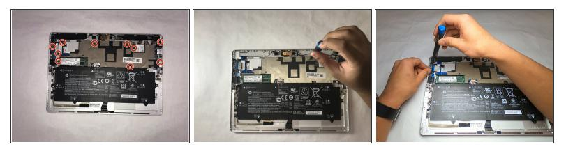
• Remove ten 2.7mm screws using the Phillips #0 screwdriver.
