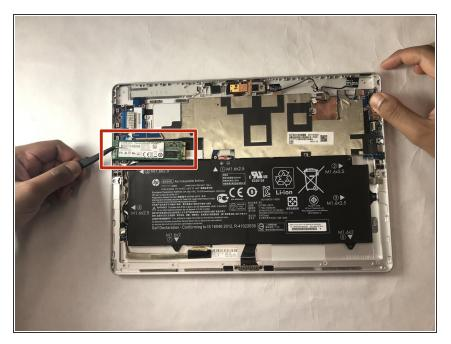
Detach the SSD from motherboard by pulling it to the left using tweezers.
