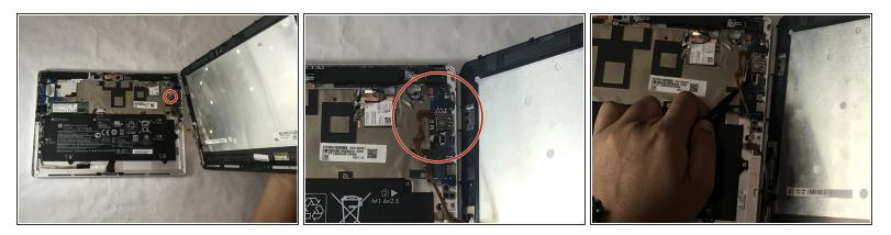
• Detach flex cable from motherboard using tweezers.
