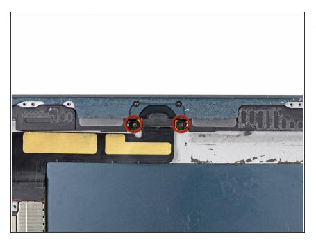
Remove two 1.4 mm #00 Phillips screws securing the left and right speakers to the rear case.
