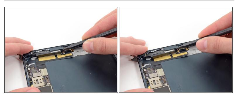
• Use the tip of a spudger to slide the right speaker slightly toward the outside of the iPad.
