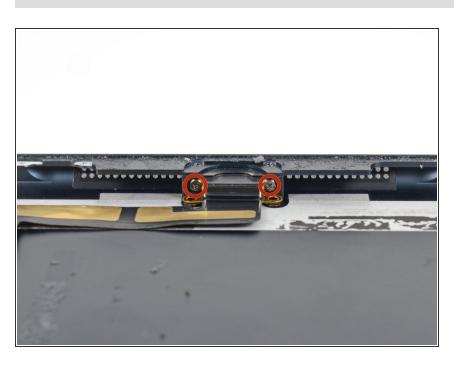
Remove two 2.8 mm Phillips #00 screws from the base of the Lightning connector. To reassemble your device, follow these instructions in reverse order.
