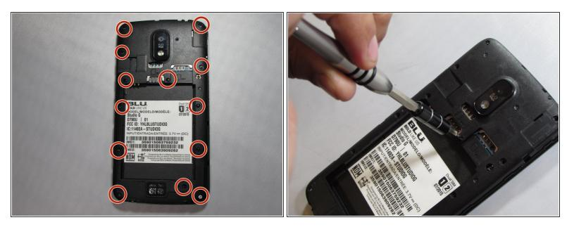
Unscrew the 13 Phillips #0 screws from the back of the phone.
