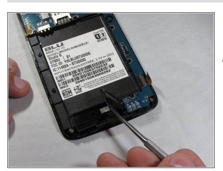
Locate the speaker on the bottom of the device and slowly pry upwards and to the right as its wired to the motherboard.
