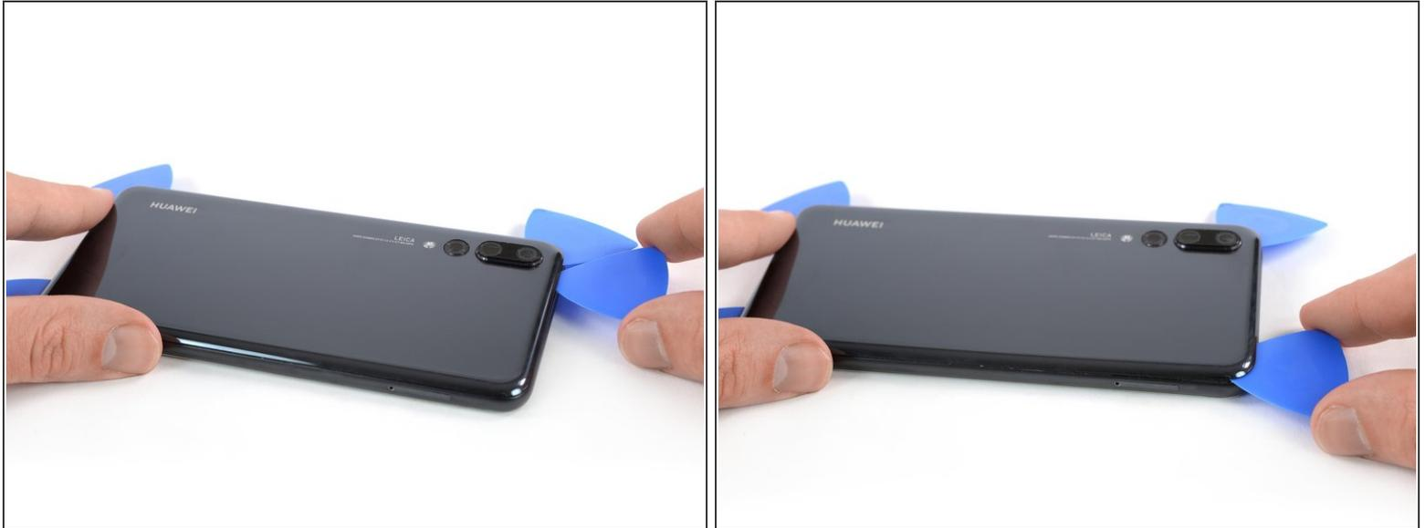
**i** In case you're having trouble to cut the adhesive, reapply the iOpener for another minute to loosen it.
