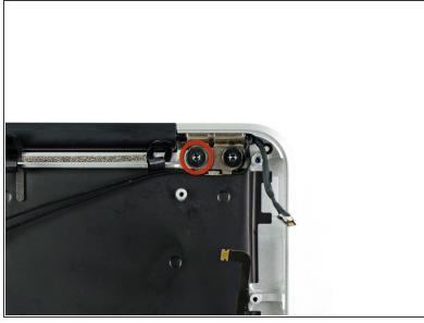
Remove the inner 4.9 mm T8 Torx screw securing each display hinge to the upper case (two screws total).
