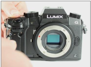
• Remove the indicated silver 5.0mm long screw from under the front cover using a Phillips PH0 screwdriver.
