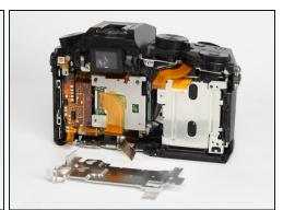
Use a PH0 Phillips screwdriver to remove the 3 indicated red 3.0mm screws from heat sink shield, then remove the heat sink.
