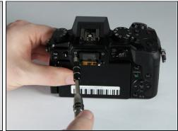
• Remove the viewfinder eye cup by pulling up and out from the bottom to separate the locking clips from the camera.
