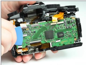
• Remove the 3 indicated flex cables from the bottom of the mainboard.
