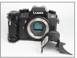
• Remove the front grip from the camera by pulling it forward and out.
