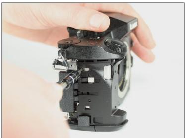
• Remove the indicated black 4.0mm long screw from the side under the front cover using a Phillips PH0 screwdriver.
