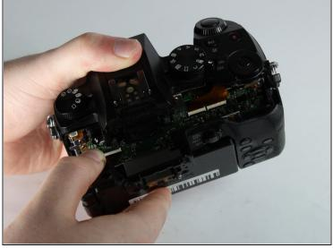
• Use an iFixit opening tool (or similarly long and thin object) to insert into the gap between the two camera halves and pry the camera apart from the top.
