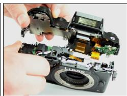
• Lift the top unit away, separating it from the rest of the unit.
