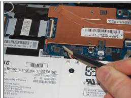
• Use the spudger to pry underneath the cable and gently lift the connector up.
