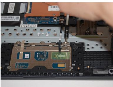
• Remove the three 2.3mm screws along the top of the trackpad using a Phillips #00 screwdriver.
