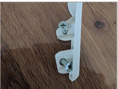
Remove these two pins that hold the plastic shell on
