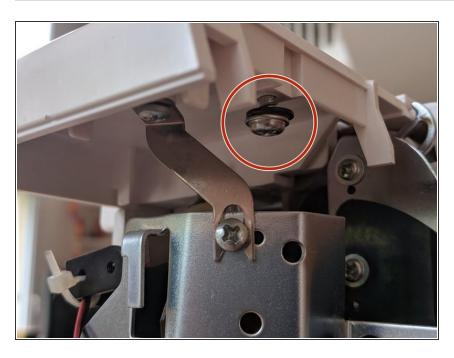
Remove this screw completely. This will allow you to remove the plastic cover
