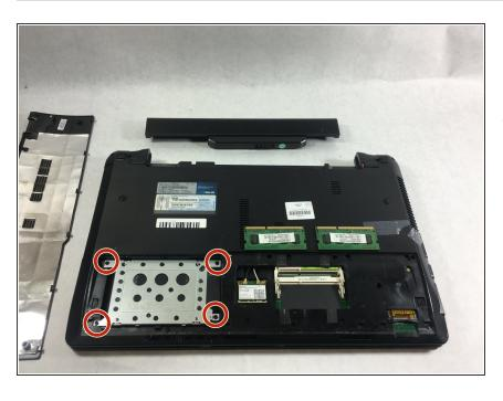
Remove the four 3mm Phillips #0 screws holding the hard drive in place.
