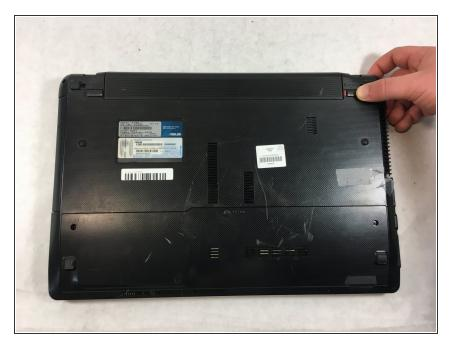
Slide the lock on the right side of the battery to the right. If done correctly the slider will stay in place and there will be a red indicator.
