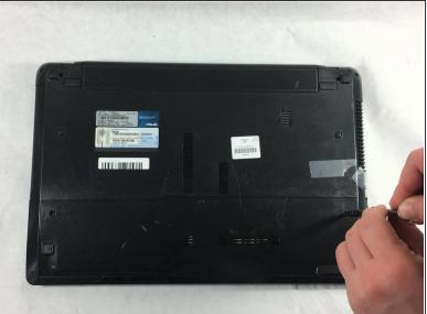
Remove the two 4mm Phillips #0 screws located on the opposite ends of the laptop.
