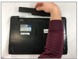
Slide the other sliding lock on the left side of the battery to the left, and with your other hand slide the battery out from the laptop.
