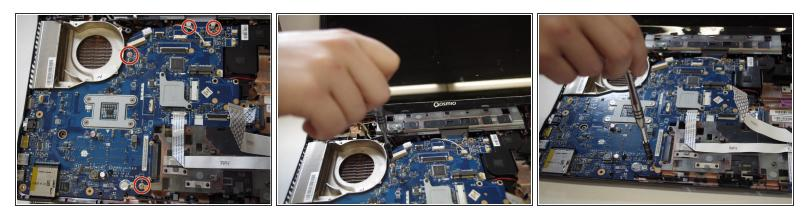
• Using a Phillips #00 screwdriver, remove the four screws securing the motherboard to the laptop.
