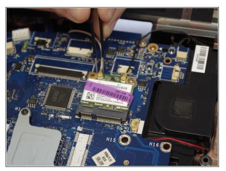
• Detach the two coaxial connections from the wifi chip.
