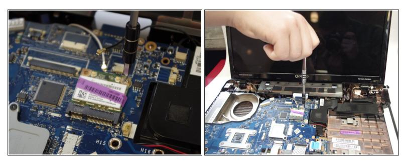
• Using a Phillips #00 screwdriver, remove the two screws from the wifi chip.
