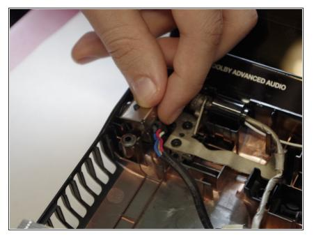
Remove the 4-pin connector housing by gently wiggling it back and forth.
