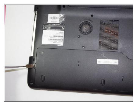
• Using a spudger or plastic opening tool, pry off the service panel.
