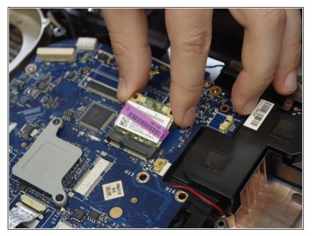
• Remove the wifi chip by pulling it out of the PCIe slot.
