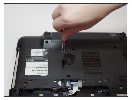
Using a Phillips #00 screwdriver, remove the optical drive retaining screw.
