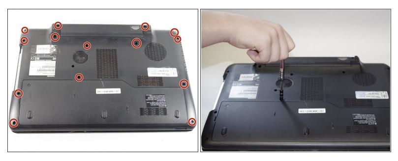
Using a Phillips #00 screwdriver, remove all the remaining fourteen screws from the bottom case of the laptop.
