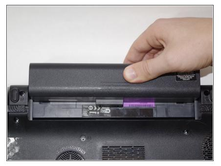
• Pull the battery straight out of its slot to remove it.
