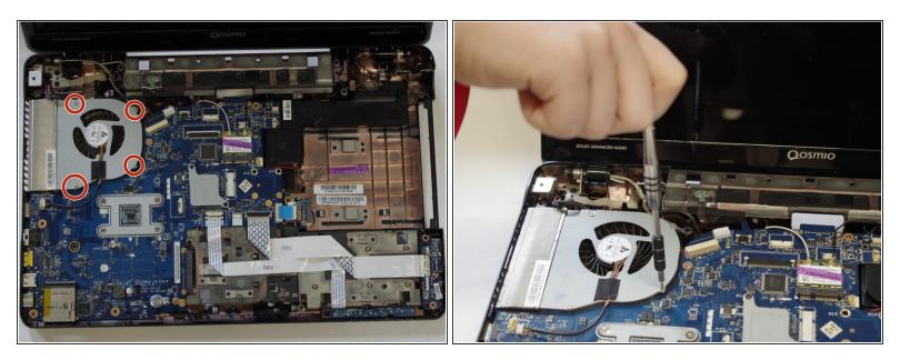
• Using a Phillips #00 screwdriver, remove the four screws securing the fan assembly to the laptop.
