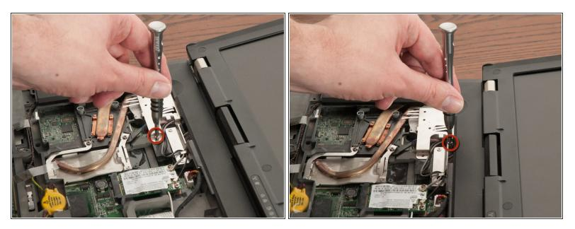
unscrew the first two screws of the shielding
