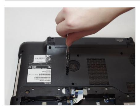
Using a Phillips #00 screwdriver, remove the optical drive retaining screw.
