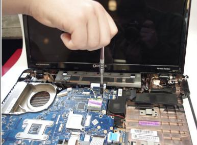
Using a Phillips #00 screwdriver, remove the two screws from the wifi chip.
