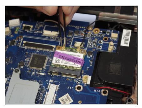
Detach the two coaxial connections from the wifi chip.
