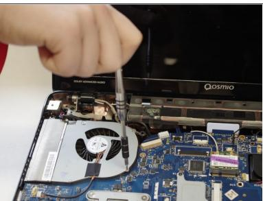
• Using a Phillips #00 screwdriver, remove the four screws securing the fan assembly to the laptop.
