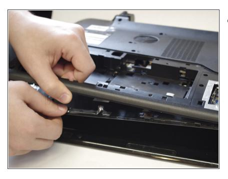
Separate the two halves of the base of the laptop.
