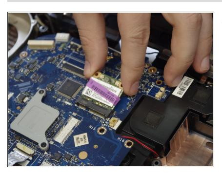
Remove the wifi chip by pulling it out of the PCIe slot.
