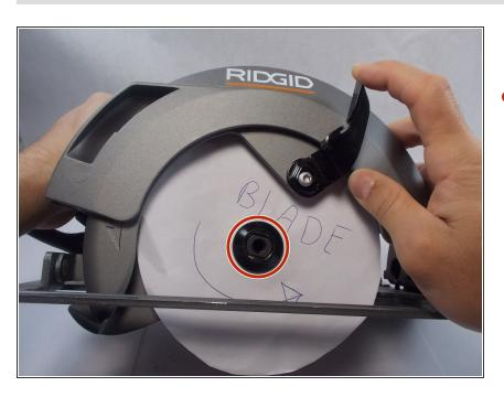
Release the spindle lock and remove the outer flange by lifting it off the output shaft.
