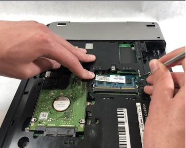
• Push outward on the two release tabs securing either side of the second RAM module.
