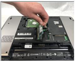
• Lift the stick of RAM upward away from the motherboard.
