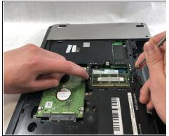
• Push outward on the two release tabs securing either side of the top RAM module.
