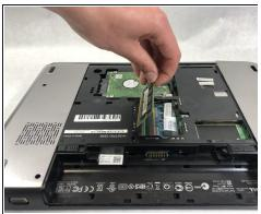
• Lift the top stick of RAM upward away from the motherboard.
