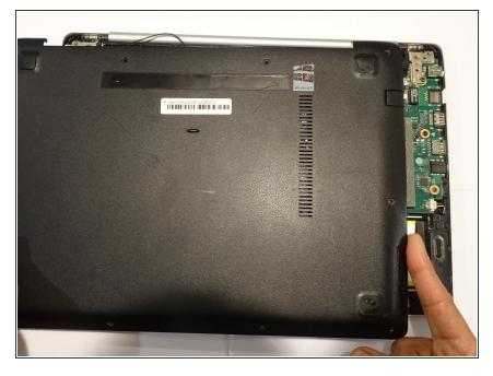
Carefully pry open the back cover from the laptop and place it to the side.
