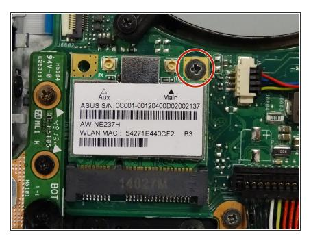
Remove the 5mm screw from the module using the Phillips PH1 screwdriver.
