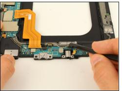
• Pry up the two coaxial cables joining the daughterboard to the motherboard.
