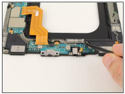
Use a spudger to pry up four press fit connectors from the lower board containing the charging port.
