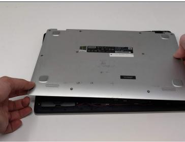
Use the nylon spudger to loosen the back cover from the back of the device.
