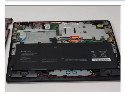
For safety reasons, disconnect the wires connecting the battery to the motherboard with the nylon spudger.
