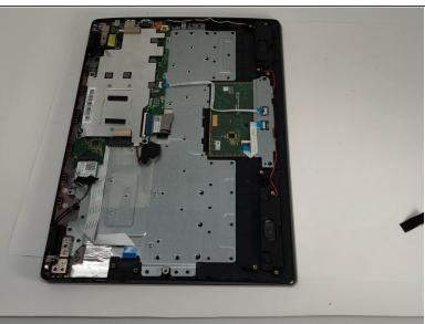
• Lift the USB/Headphone Jack PCB off of the board gently and put it to the side.
