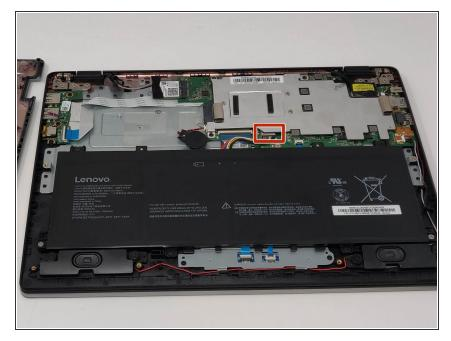
For safety reasons, disconnect the wires connecting the battery to the motherboard with the nylon spudger.
