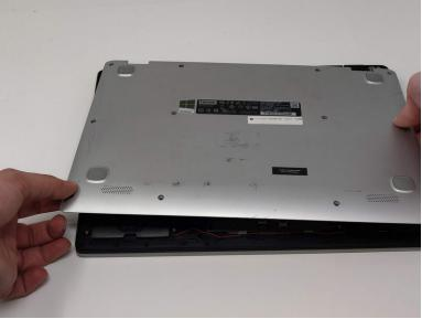
• Use the nylon spudger to loosen the back cover from the back of the device.
