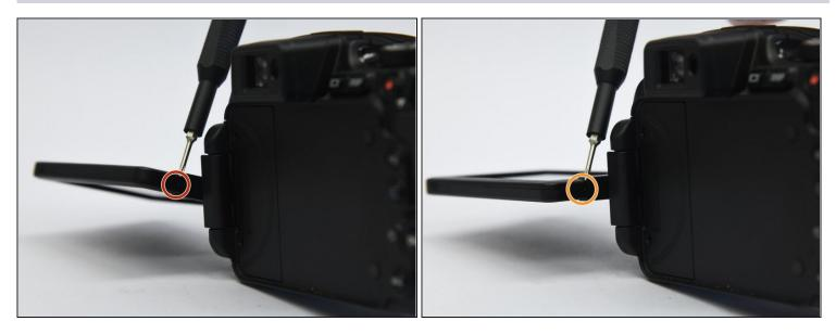
• Use a Phillips screwdriver to remove the two 3.5mm screws on both sides of the side of the screen.
