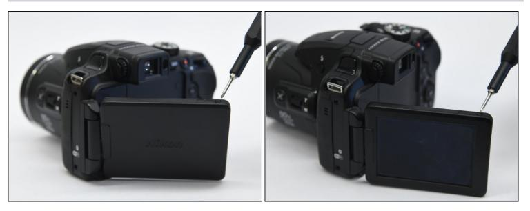
• Use a Phillips screwdriver to remove the two 3.5mm screws at the top and bottom of the LCD Screen.
