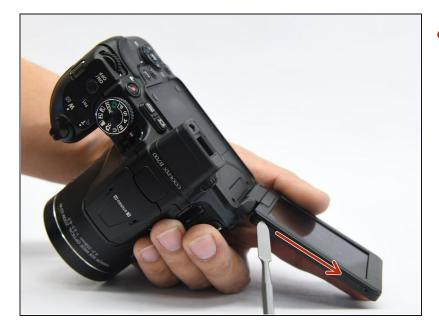
• Use to metal spudger to pry open the LCD cover. Then slide it down the length of the screen until the cover comes apart.
