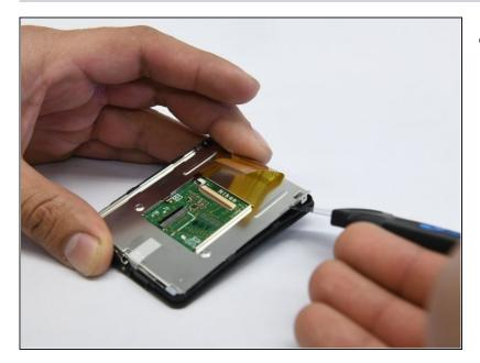
• Use the jimmy and slide it in between the LCD screen and lift out the LCD Screen.
