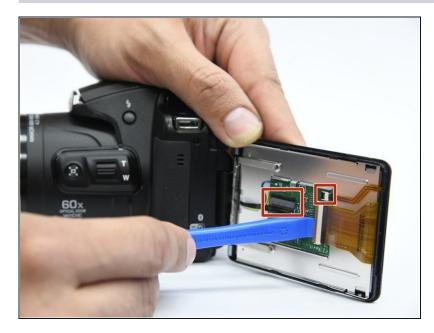
• Use the pry tool and slide it under the black tab and lift up gently. Do this again for the other two ZIF tabs.
