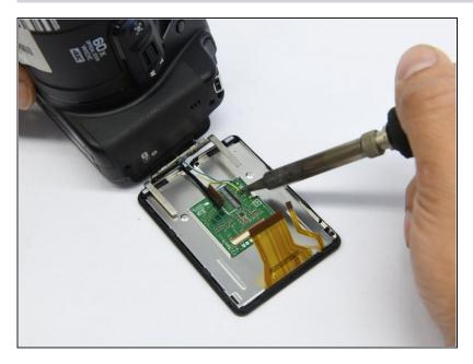
• Use the <u>solder gun</u> and desolder the yellow and blue wires.
