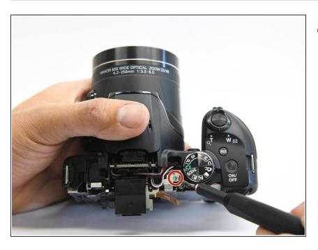
On the top of the camera, remove the 6mm screw.
