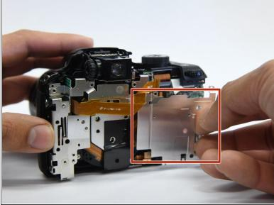
• Gently lift up the button assembly to slide the bracket out.
