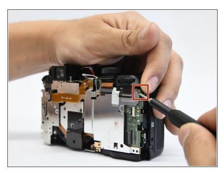
Lift the button assembly gently to give access to remove the 4mm screw.
