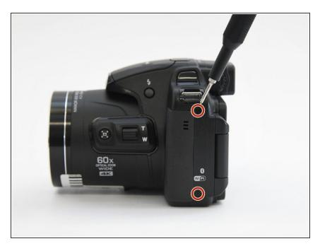
Use the Phillips screwdriver to remove the two 5.5 mm screws on the left side of the camera.
