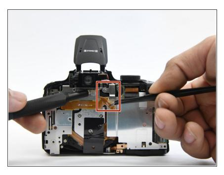
Move the ribbon out of the way to reveal the hidden screw.
