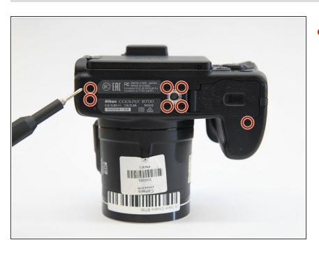
Use the Phillips screwdriver to remove seven 5.5 mm screws from the bottom of the camera.
