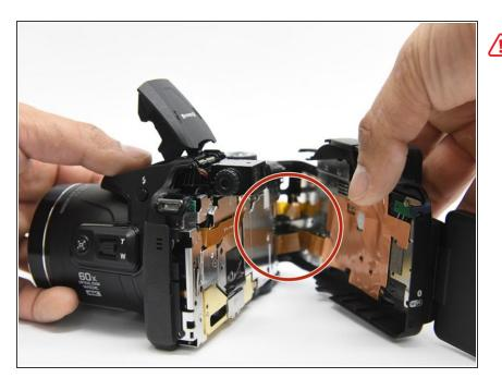
Be careful not to damage the ribbons that connect the halves together.
