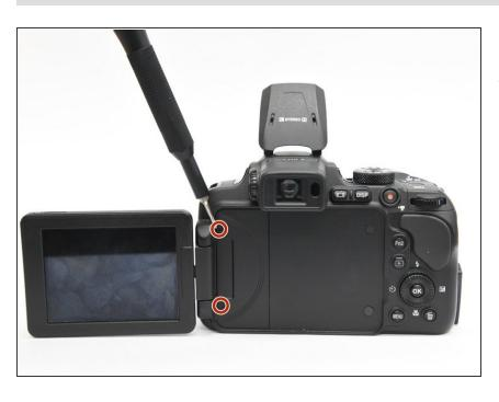
Use the Phillips screwdriver to remove the two 5.5mm screws under the LCD panel.
