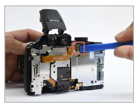
Insert the pry tool under the latch and gently lift up to remove the ribbon.
