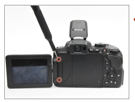
Use the Phillips screwdriver to remove the two 5.5mm screws under the LCD panel.
