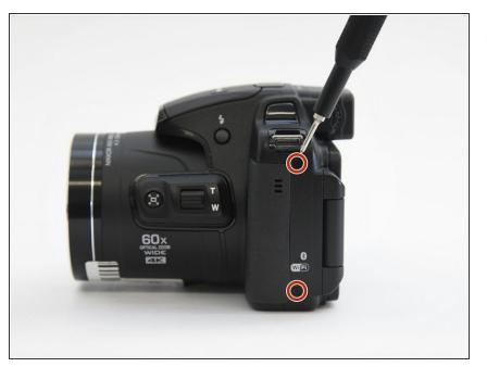
Use the Phillips screwdriver to remove the two 5.5 mm screws on the left side of the camera.
