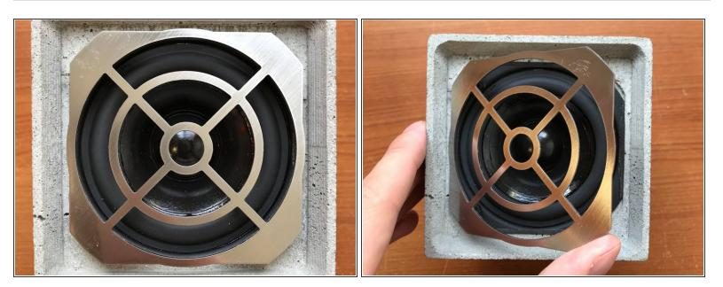
Remove the protective grille by lifting one of the four corners.
