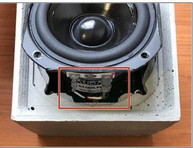
First connect the positive and negative wires, then slide the speaker in the enclosure in the right orientation
