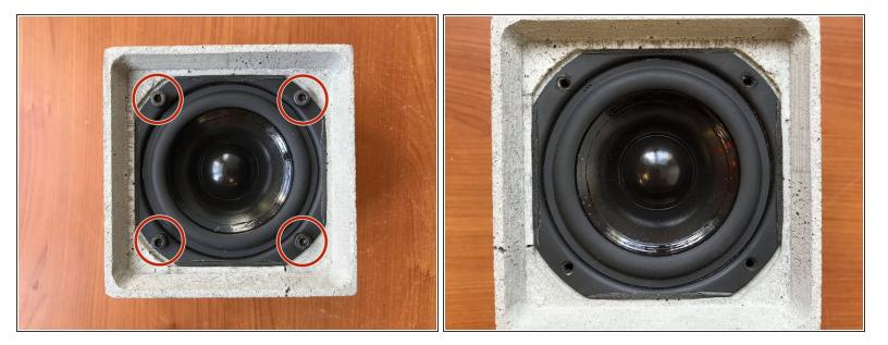
Remove the four screws using a m4 allen wrench
