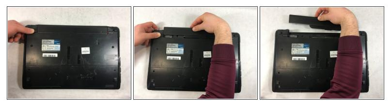
• Slide the other sliding lock on the left side of the battery to the left, and with your other hand slide the battery out from the laptop.
