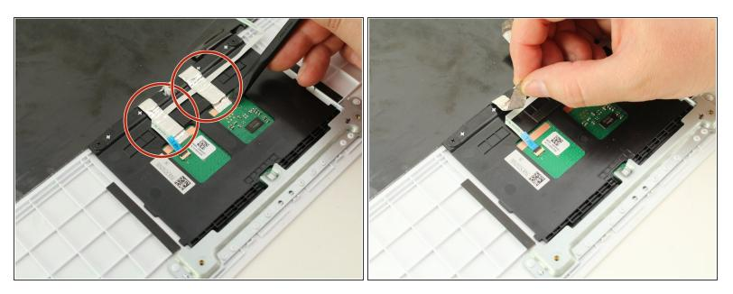
• Peel up the two pieces of foil tape holding down the trackpad.
