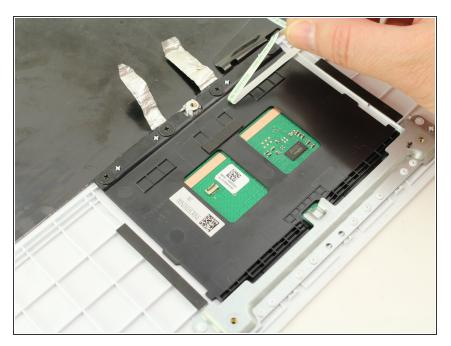
• Peel back the ribbon cable, which is adhered to the trackpad.
