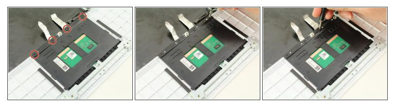
• Remove the four 2.5mm Phillips #0 screws along the top edge of the trackpad.
