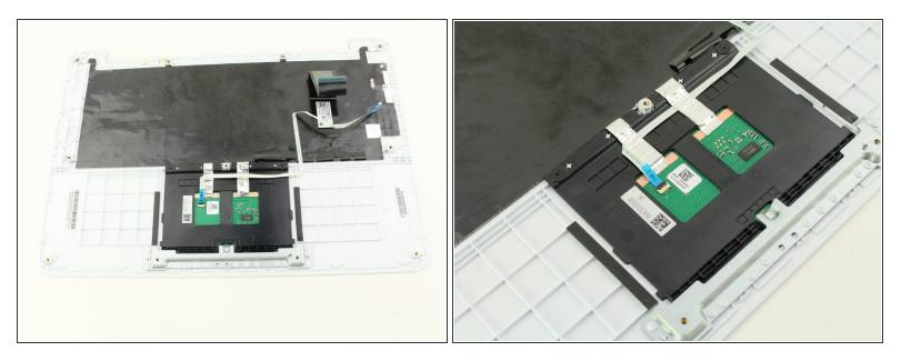
• Flip over the keyboard assembly to reveal the trackpad beneath.
