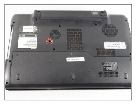
Locate the optical drive retaining screw on the underside of the laptop.
