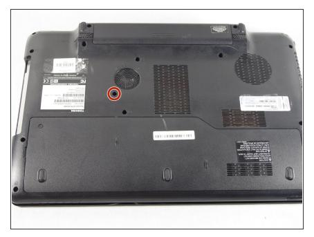
Locate the optical drive retaining screw on the underside of the laptop.
